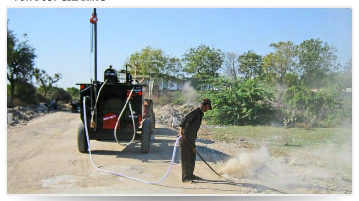
Tractor linked tyre mounted Bitumen-Emulsion Sprayer with Compressor for road dust cleaning is developed for tack / prime coat by hand spraying arrangement and intermittent spraying application with road dust cleaning also. This equipment is capable of applying uniform coating of Hot Bitumen & Emulsion on specified surface.
